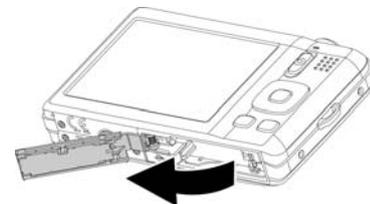
3. Insert the battery into the compartment with the terminal facing inside the camera with correct orientation as shown.
