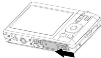
2. Unlock and open the Battery/memory card compartment at the bottom of the camera.
